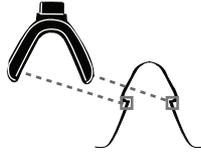
2) To detach, pull a leg of the nose piece once the leg is disengaged, the nose piece will simply rotate out.
