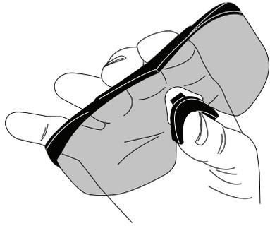
1) Align grooves of nose piece into the primary lens and squeeze together until the nose piece completely seats into the lens.
