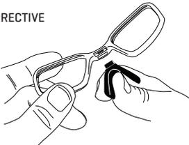
2) Fully insert the post at the top of the nosepiece into the slot of the Rx Carrier.
