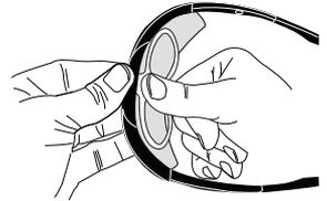
2) To remove Rx Carrier slide finger tip between Rx lens and protective lens. Grasp firmly as close to the frame as possible and pull out from frame.
