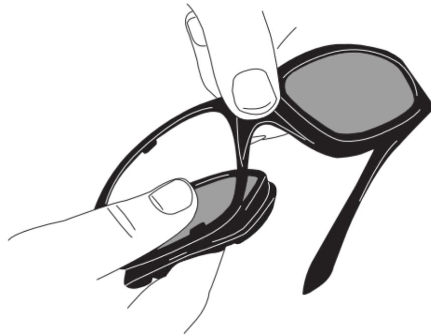
Hold the frame at the nose piece and rotate the lens from top of the frame.
